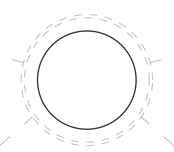
Use dotted line for **Under Mount**. Sink rim is about 1/2" (12.5 mm) revealed from the edge of the counter top opening.
